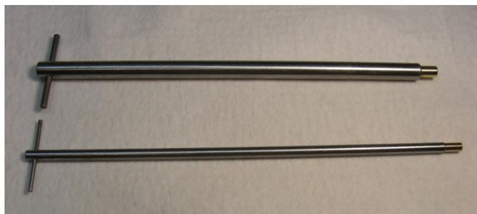
Two different size tap handles are shown. The top one is 13/32" in diameter and fits inside the Sherline spindle itself, while the smaller one at 1/4" diameter is for use with a WW collet holder. Fitted into the end of each shaft is a cut-off clock key providing the square hole for the end of the tap. (The apparent curve in the shaft is caused by the wide angle lens.)
