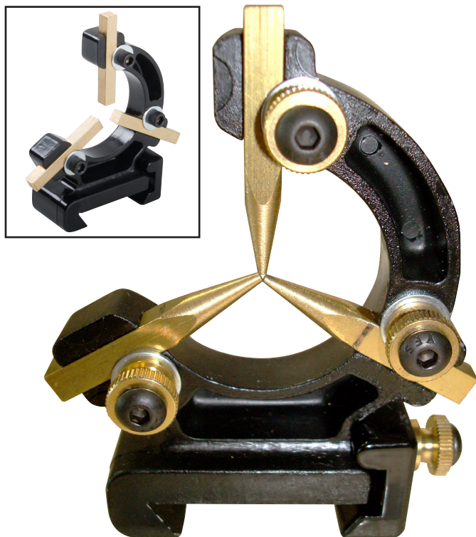
FIGURE 1—The small inset photo shows the brass blades with the square faces as they come from the Sherline factory. The large photo shows Gary Combs' modification with the tapers on the blades.
